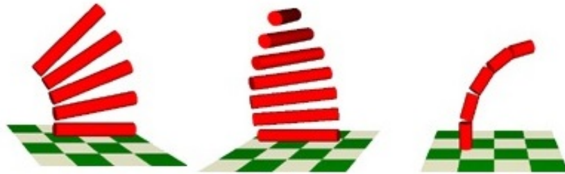
Figura 4.1: K_{11} (Splay), K_{22} (Twist) e K_{33} (Bend)[74].
